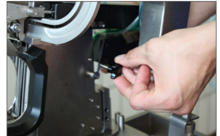
Service-friendly: knife replacement without tools
